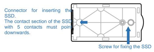
Insert the memory in the M.2 slot paying close attention to the correct orientation.
